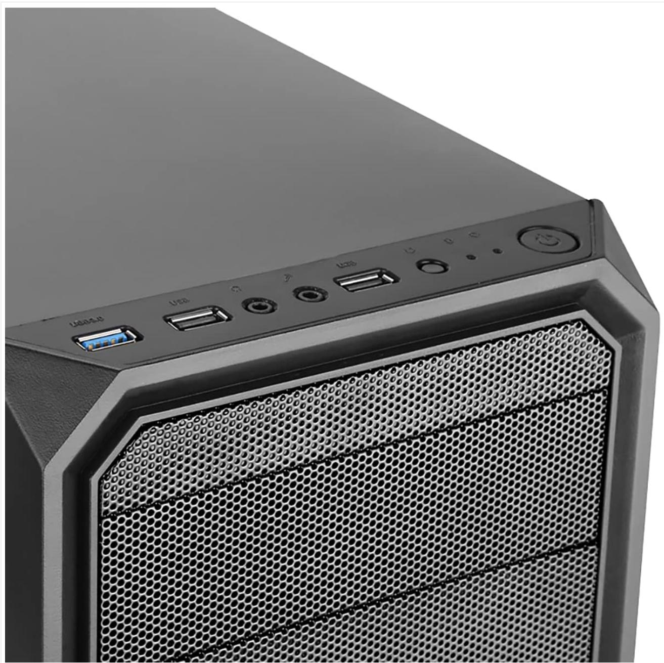
Located on the top front of the case, the I/O panel provides easy access to one USB 3.0 port, one USB 2.0 port, HD audio jacks (headphone and microphone), power and reset buttons, and a convenient SD/TF card reader.
