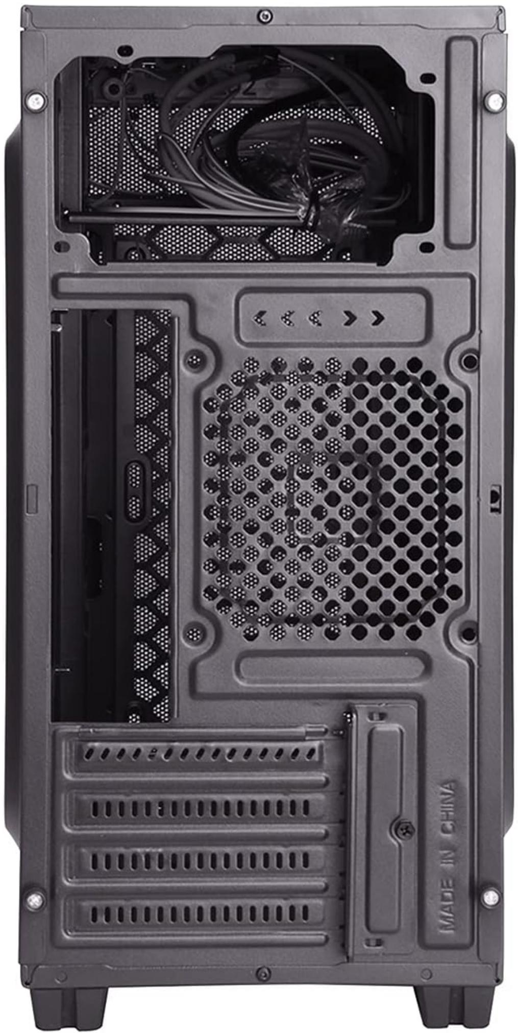
The rear panel features the bottom-mounted power supply unit (PSU) bay, expansion slots for graphics cards and other add-in cards, and a rear fan mounting area for exhaust.
