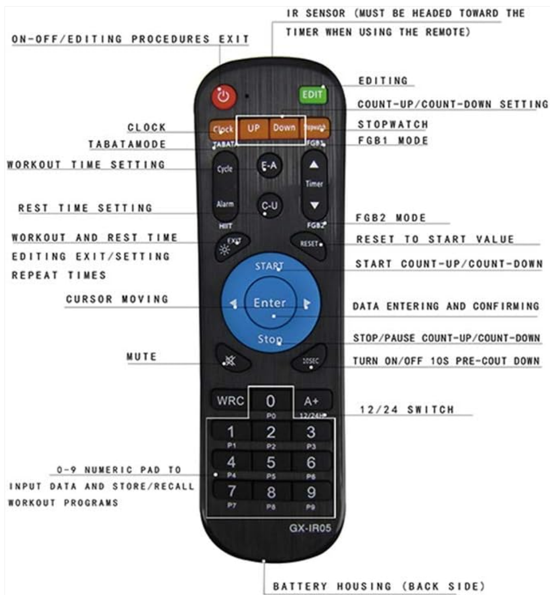
Figure 4: GX-IR05 Remote Controller Button Functions.
