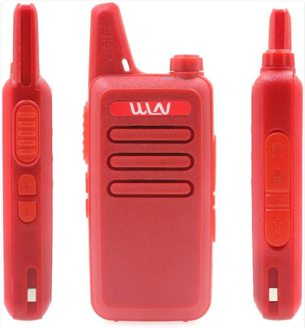
Image: Front, left, and right side views of the WLN KD-C1 radio, highlighting the integrated antenna, speaker/microphone, channel selector, volume/power knob, and side buttons.
