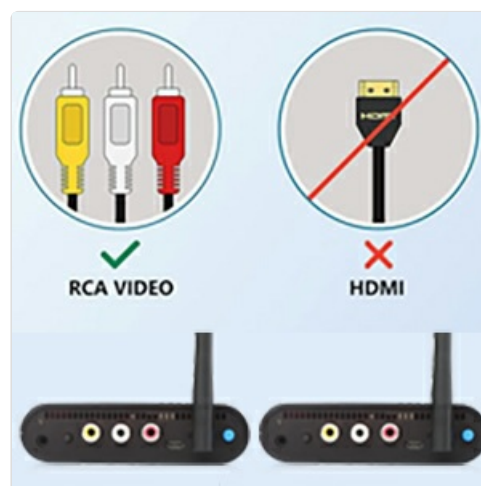
Figure 2.4: RCA connection is required.
