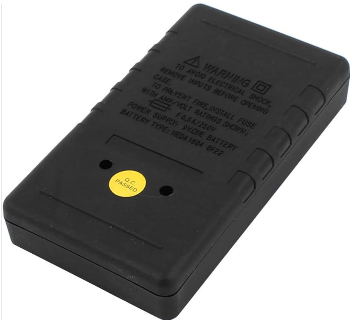
Figure 2: Back view of the Aexit DT-830B Digital Multimeter showing the battery compartment and safety warnings. This image shows the rear casing of the DT-830B Digital Multimeter. A prominent warning label is visible, advising users to remove inputs before opening the case to avoid electrical shock and to install a 0.5A/250V fuse to prevent fire. The power supply requirement of a 9V (6F22) battery is also stated. The battery compartment is located on the back, typically secured by screws.
