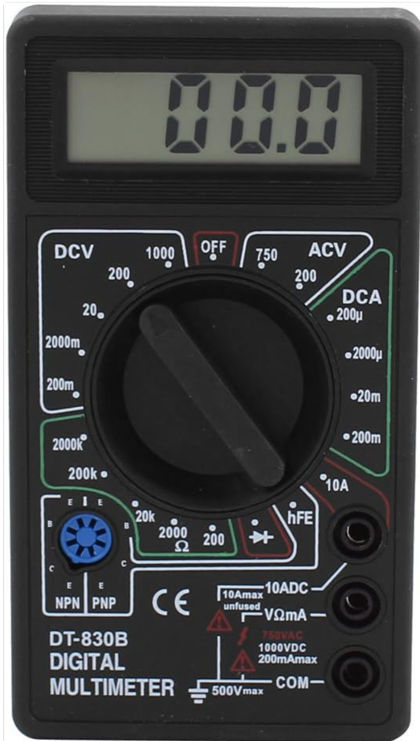
Figure 1: Front view of the Aexit DT-830B Digital Multimeter showing the LCD display, rotary switch, and input jacks. Key components visible include the 3 1/2 digit LCD screen at the top, the central rotary switch for function and range selection, and the input jacks (VΩmA, 10ADC, COM) at the bottom right. The various measurement ranges for DCV, ACV, DCA, Resistance, Diode, and hFE are clearly marked around the rotary switch.
