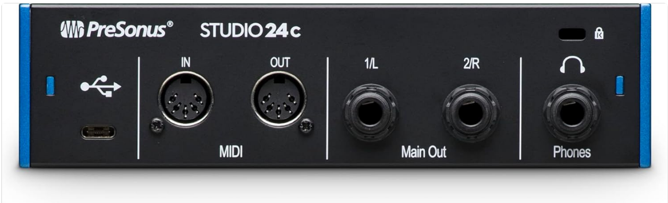
Figure 5: Rear view of the Studio 24c with labeled connections.
