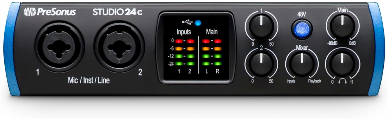
Figure 4: Front view of the Studio 24c with labeled controls.
