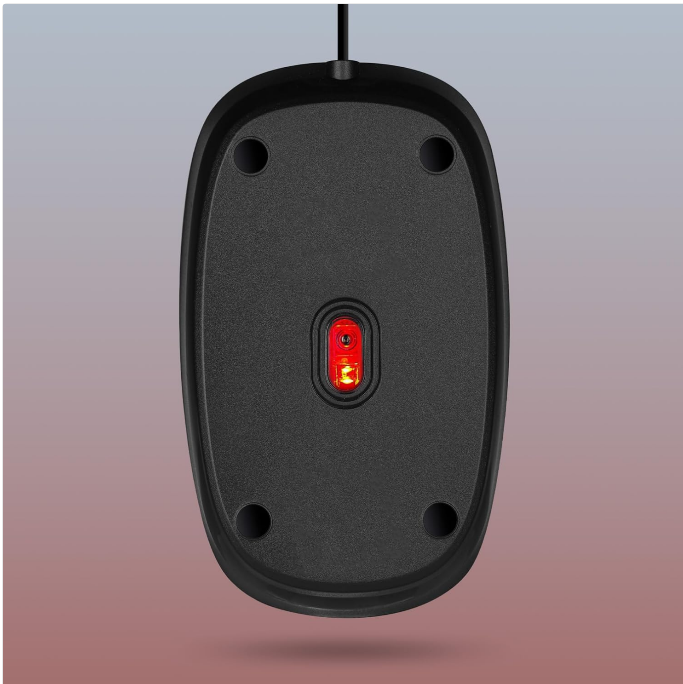
Figure 6: The underside of the mouse, showing the optical sensor. Keep this area clean for best performance.
