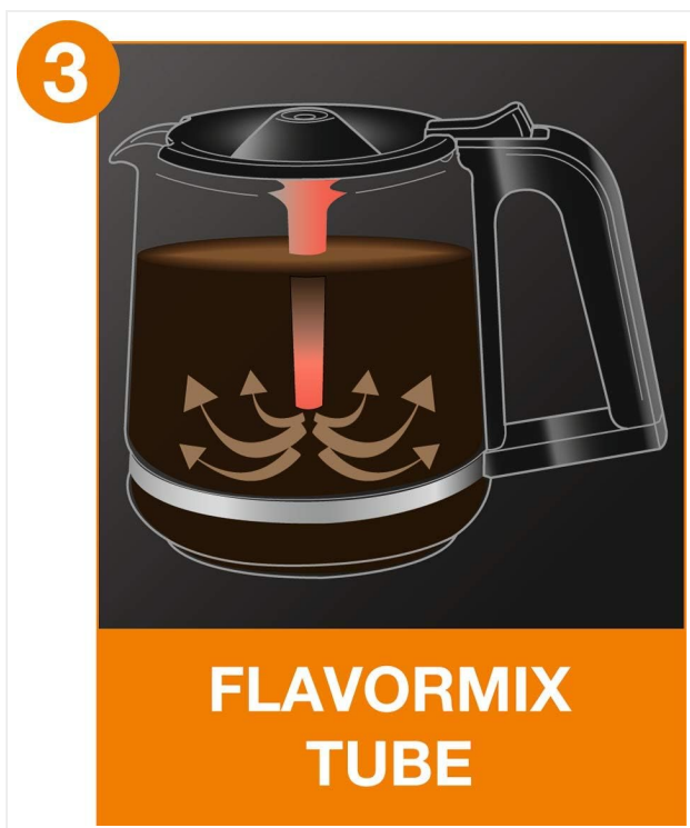
Figure 6: Diagram illustrating the Flavor Mix Tube within the carafe, which circulates the brewed coffee to ensure a consistent and balanced flavor throughout the entire pot.
