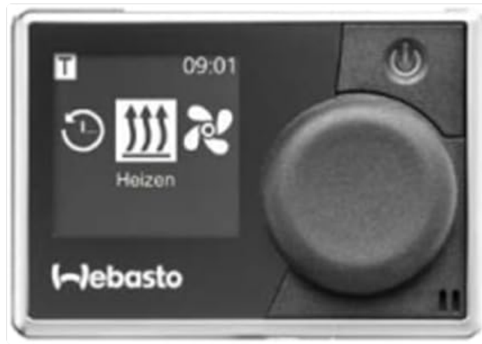
Figure 1: Front view of the Webasto MultiControl Timer. The display shows the current time (09:01) and icons for heating (Heizen) and fan operation. A rotary knob and power button are visible on the right.
