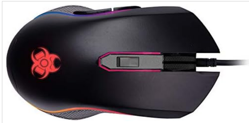
Image 5.1: Top-down view of the gaming mouse, clearly showing the scroll wheel, the DPI adjustment button behind it, and the left and right click buttons. The Tracer logo with RGB lighting is visible at the rear.
