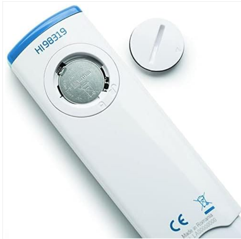
Figure 3.1: View of the battery compartment on the back of the HI98319.
