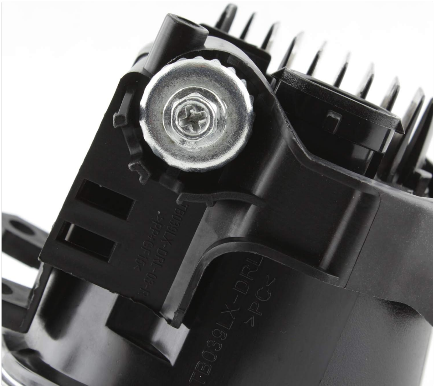
Figure 4.1: Detail of the fog light mounting point.
