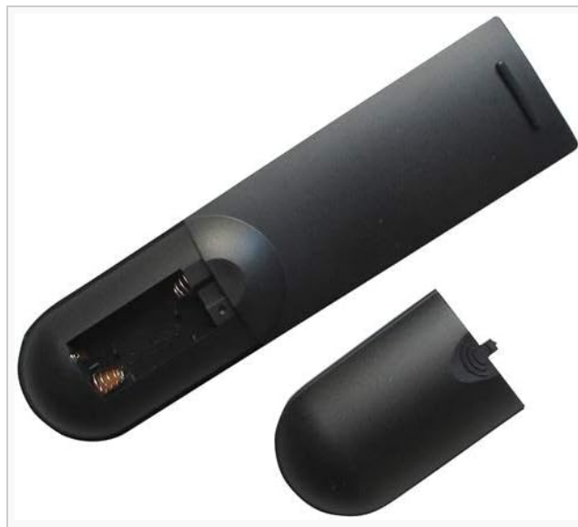
Figure 3.1: Back view of the remote control with the battery compartment open, illustrating where to insert the two AAA batteries.
