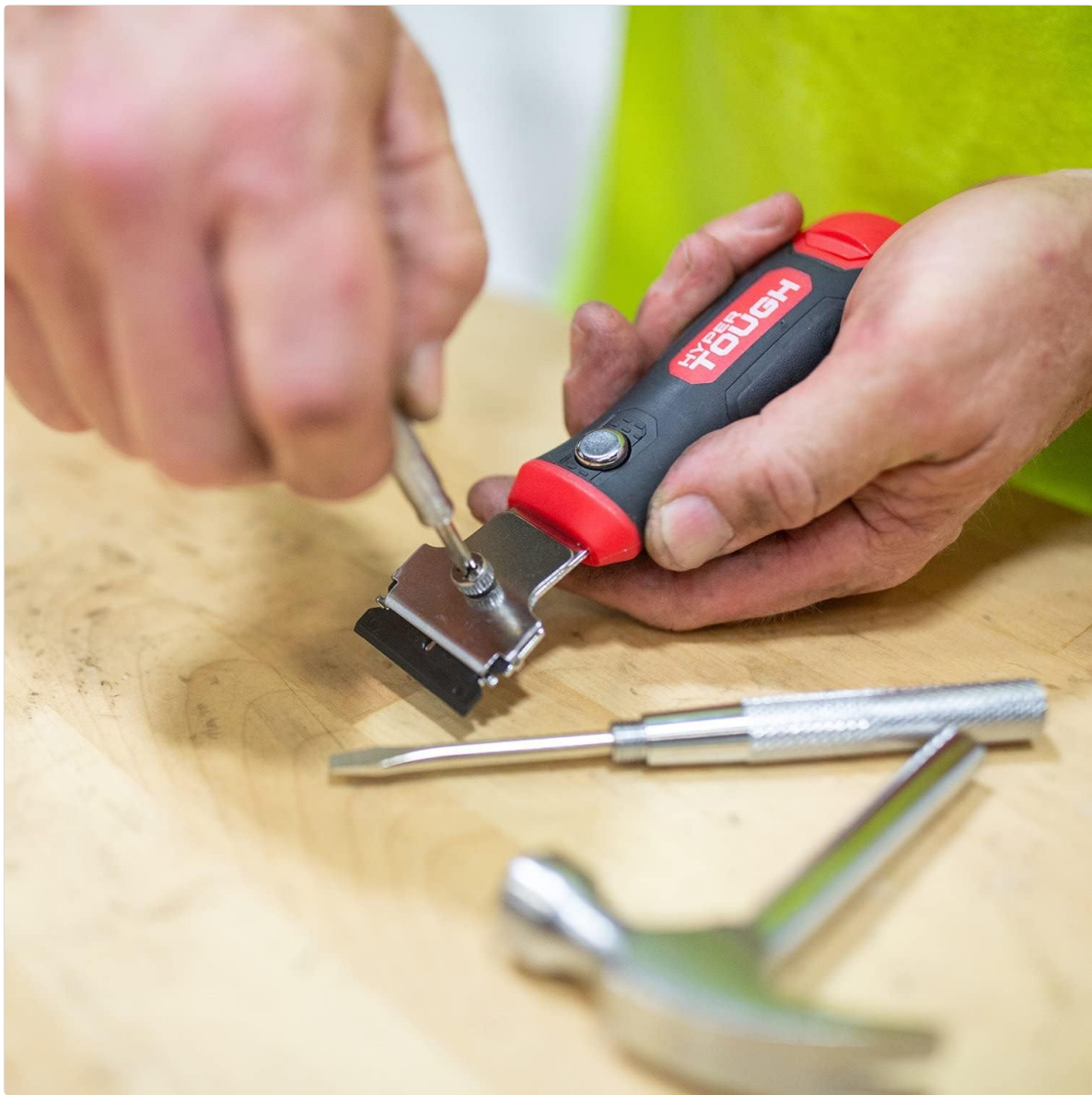
Figure 3: Securing the blade with the tightening screw using a screwdriver.
