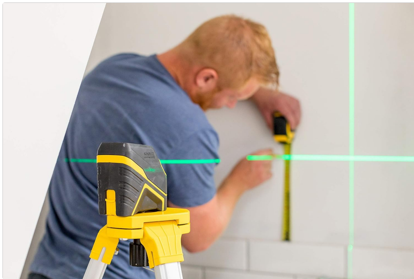
Figure 5: Laser level in operation, projecting precise green cross lines for measurement.
