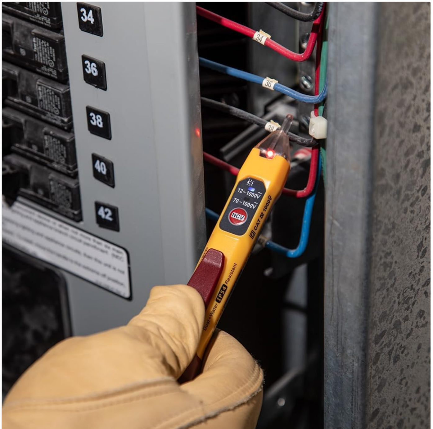
Image: A hand holding the NCVT2P tester near wires inside a circuit breaker panel. The red LED is illuminated, indicating the presence of voltage.
