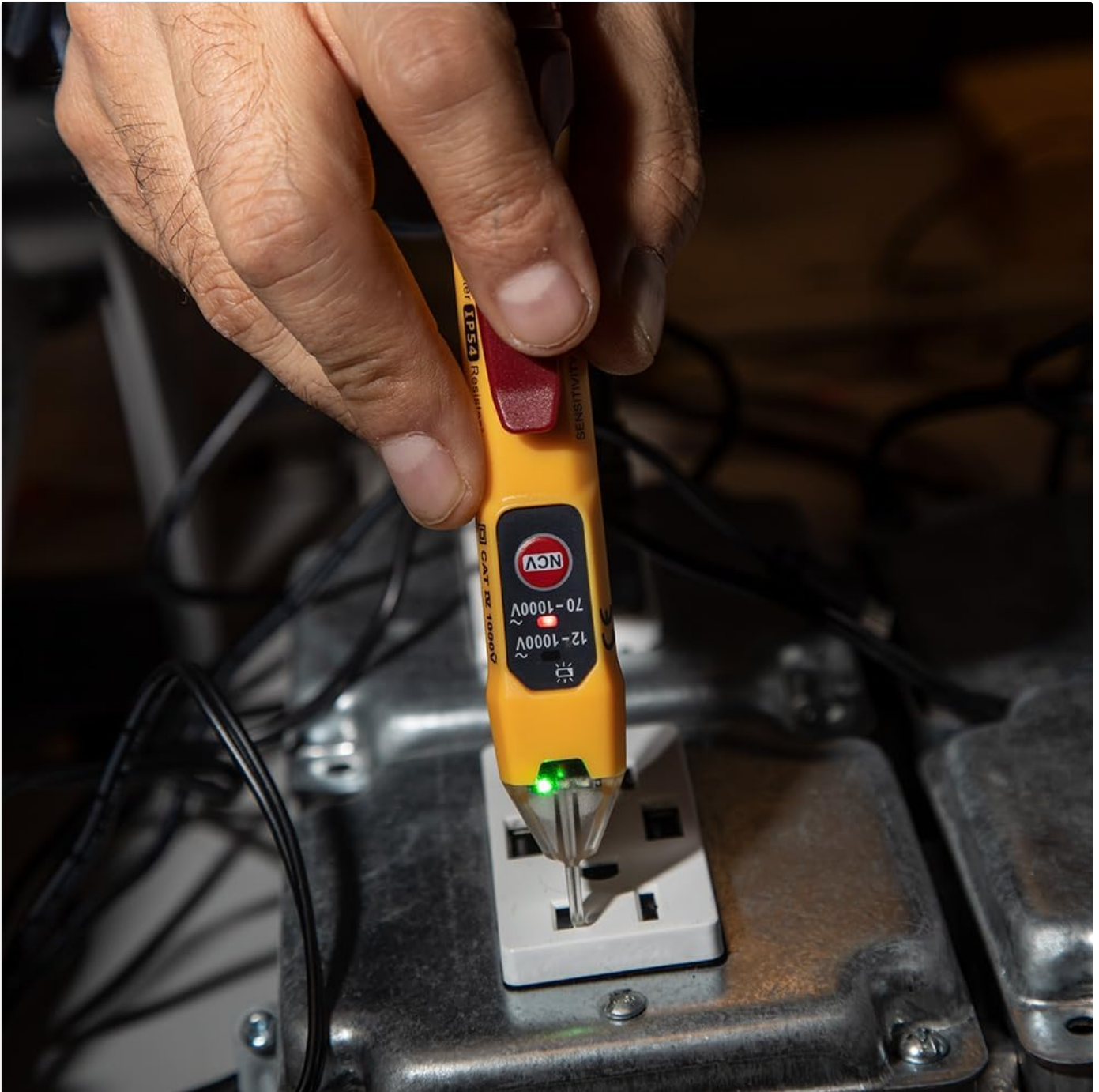
Image: A hand holding the NCVT2P tester near an electrical outlet. The green LED is illuminated, indicating no voltage detected at this point.
