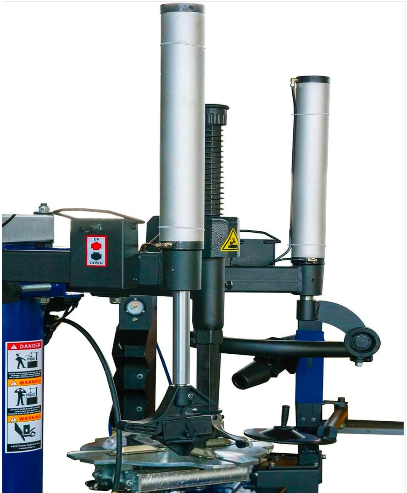
Image 4: Helper arm. This auxiliary arm assists in managing tire beads, particularly for stiff or low-profile tires.
