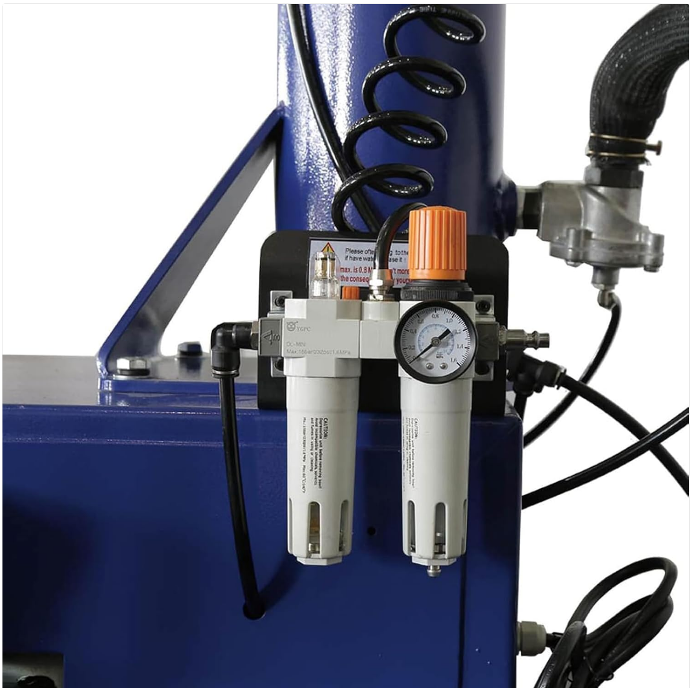
Image 1: Air regulator and filter unit. This component manages the air pressure and filters the air supply to the tire changer.
