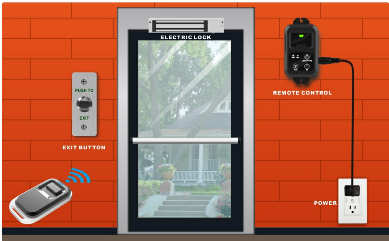
Figure 8: An overview of the access control system components and their placement relative to a door.
