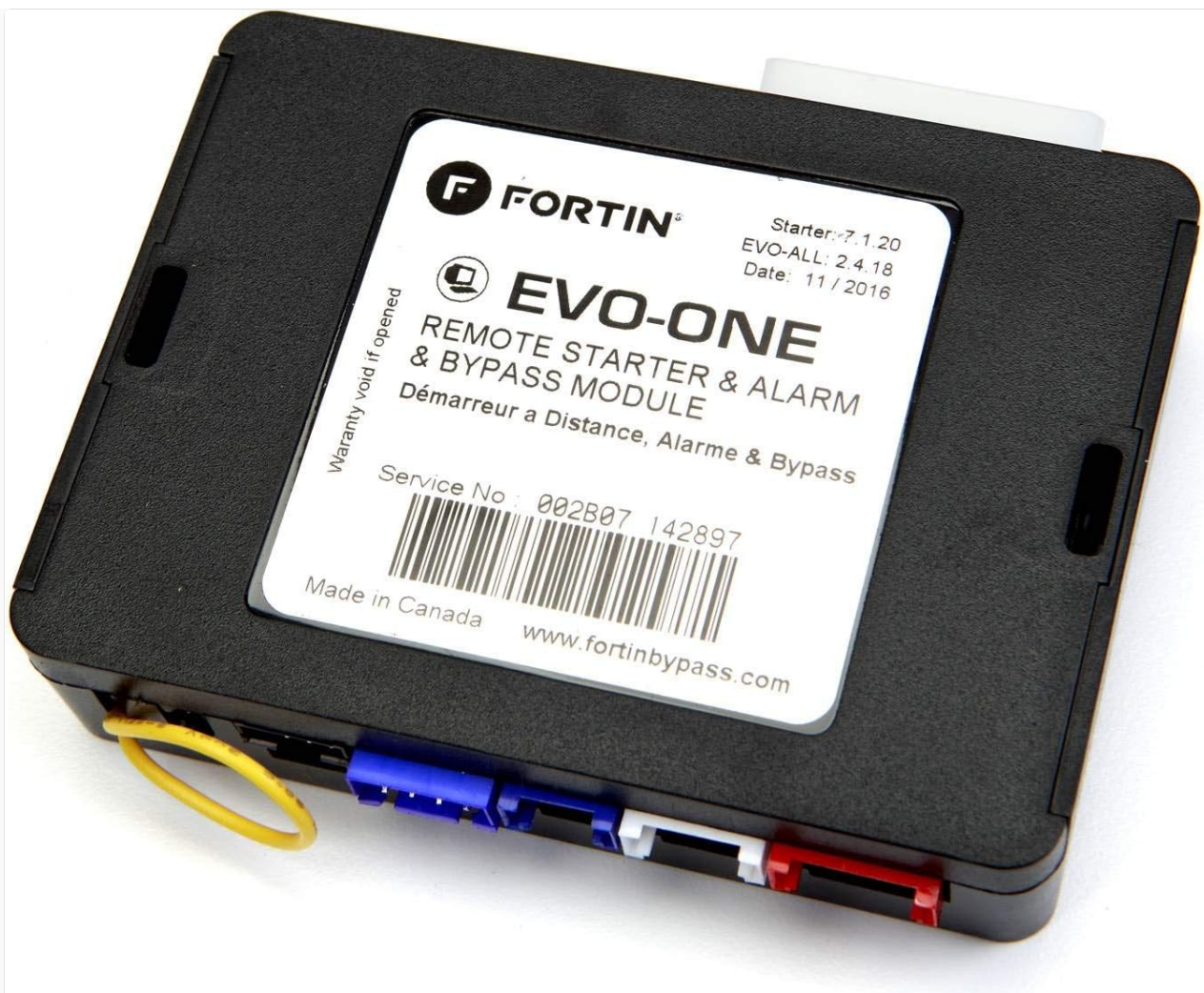
Figure 3.1: Top view of the Fortin EVO-ONE module, showing the product label with model information, serial number (e.g., 002B07 145086), and manufacturer website www.fortinbypass.com .
