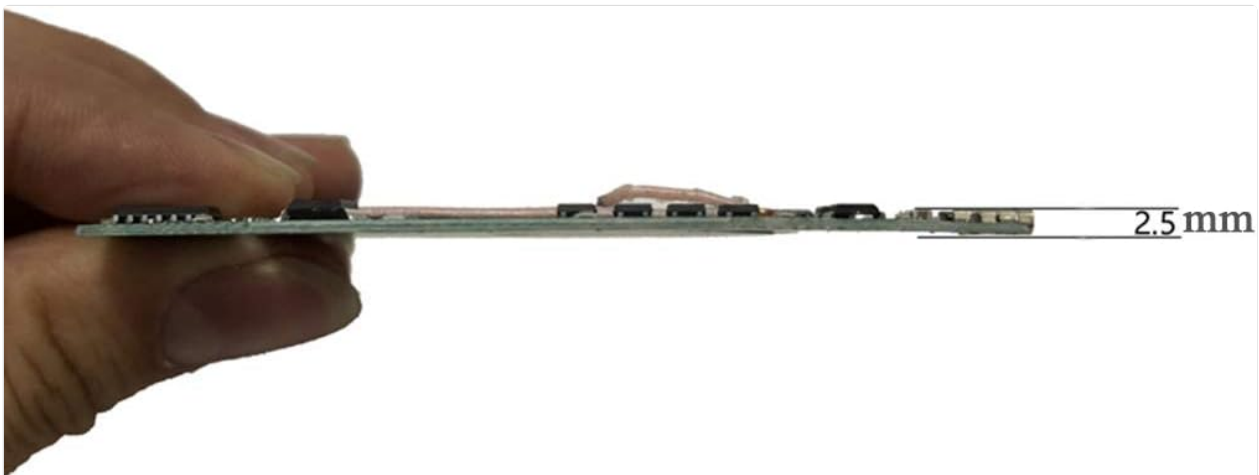
Figure 3: Side profile of the Taidacent Wireless Charger Transmitter Module, illustrating its ultra-thin 2.5mm design.
