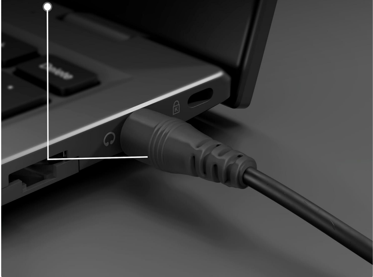
Image: Connecting the 3.5mm AUX input cable to a laptop's audio jack.
