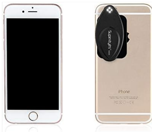
Image 3.1: The Supereyes S003 microscope and its magnetic metal plate.
