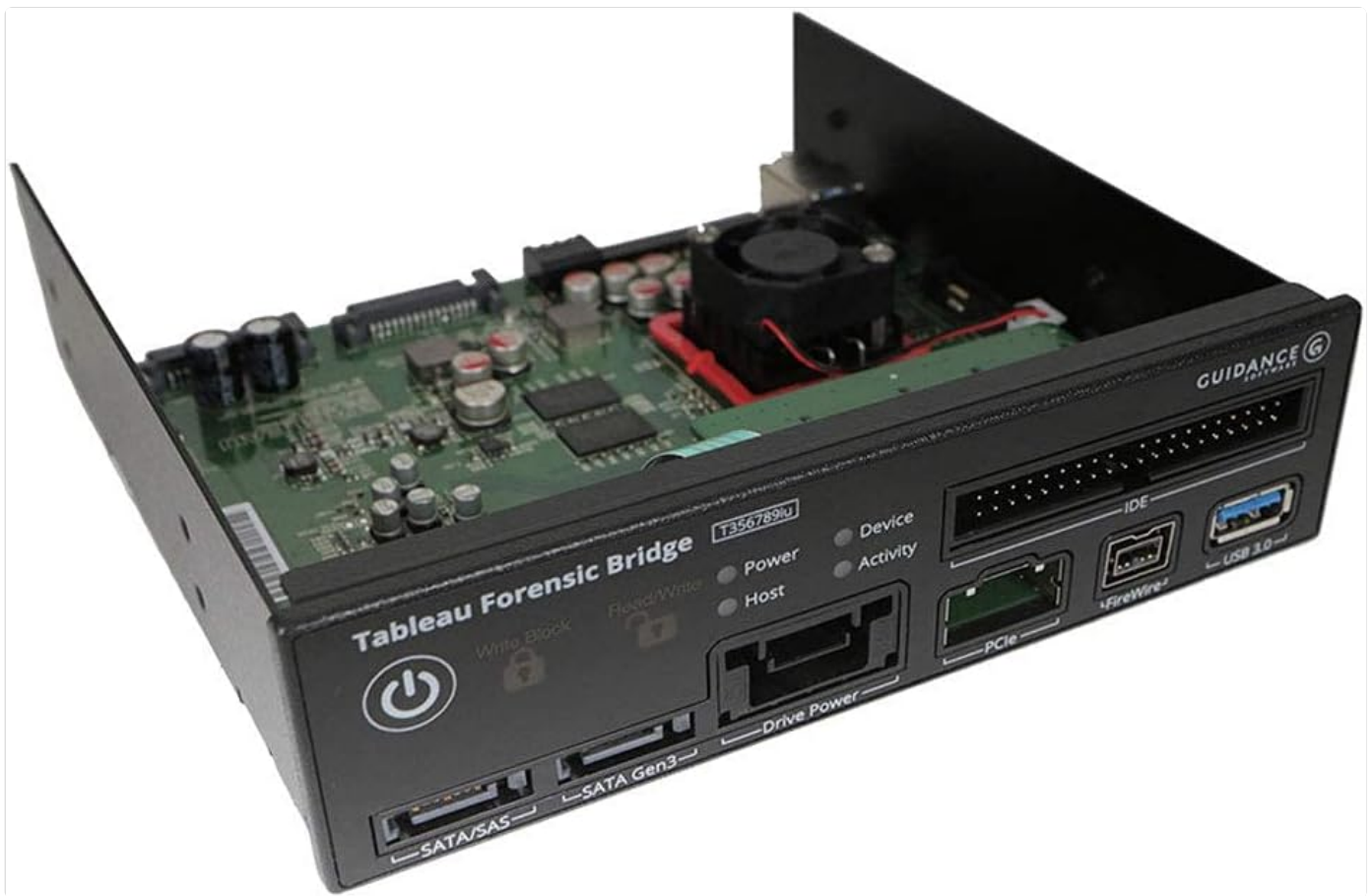
Figure 4: Internal view of the Tableau T356789iu, showing the circuit board and various connectors.
