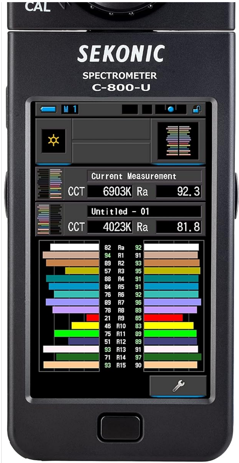
Image: The C-800-U display showing Correlated Color Temperature (CCT) and Color Rendering Index (Ra) values.
