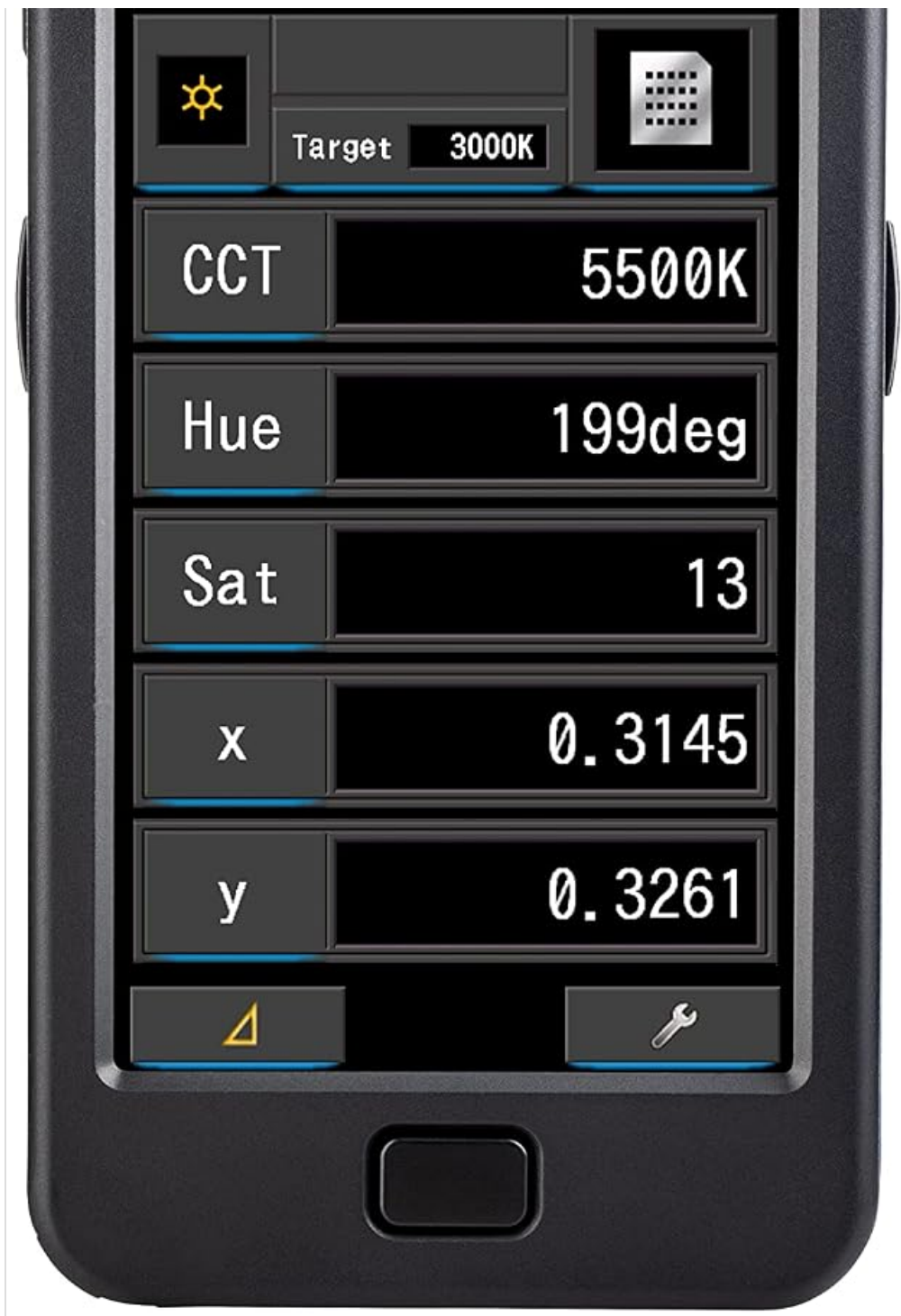
Image: The C-800-U display showing CCT, Hue, Saturation, and CIE 1931 x,y chromaticity coordinates.
