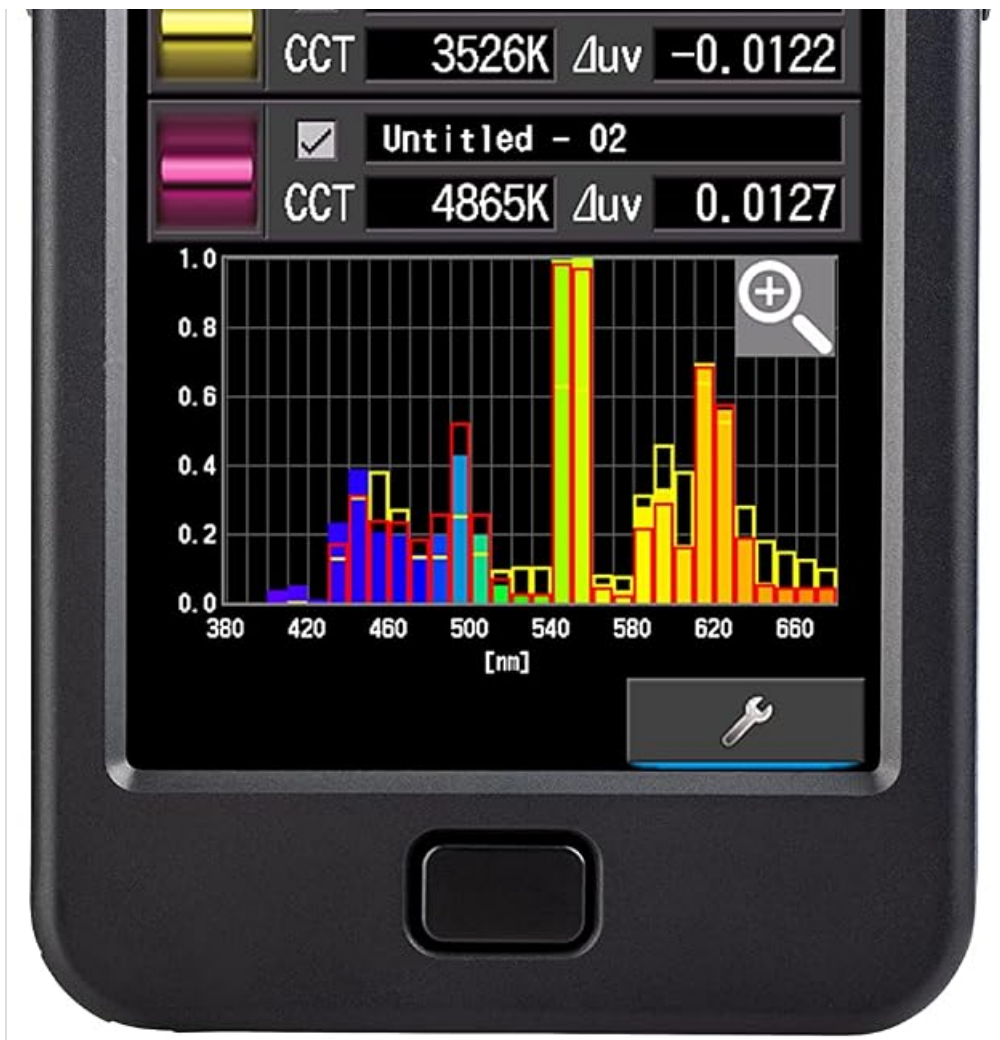
Image: The C-800-U display showing Spectral Similarity Index (SSI) and a detailed spectrum graph.
