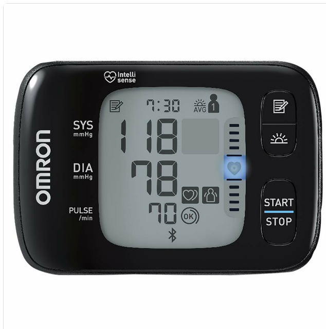
Image: A close-up view of the Omron HEM 6232T's digital display, showing blood pressure readings and various indicators.
