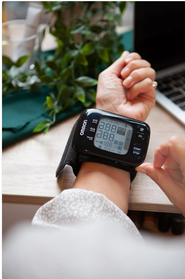
Image: A person actively taking a blood pressure reading with the Omron HEM 6232T, showing the device positioned at heart level.
