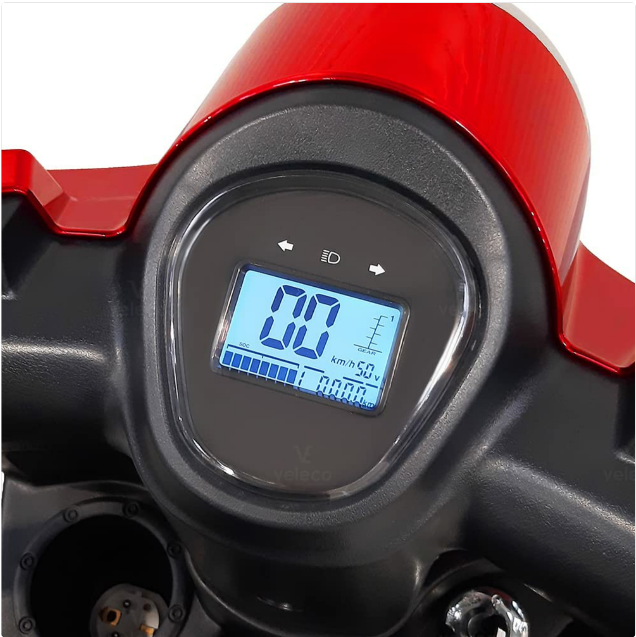
Figure 3.7: Detailed view of the digital dashboard, providing clear readings for speed, battery charge level, and turn signal indicators.
