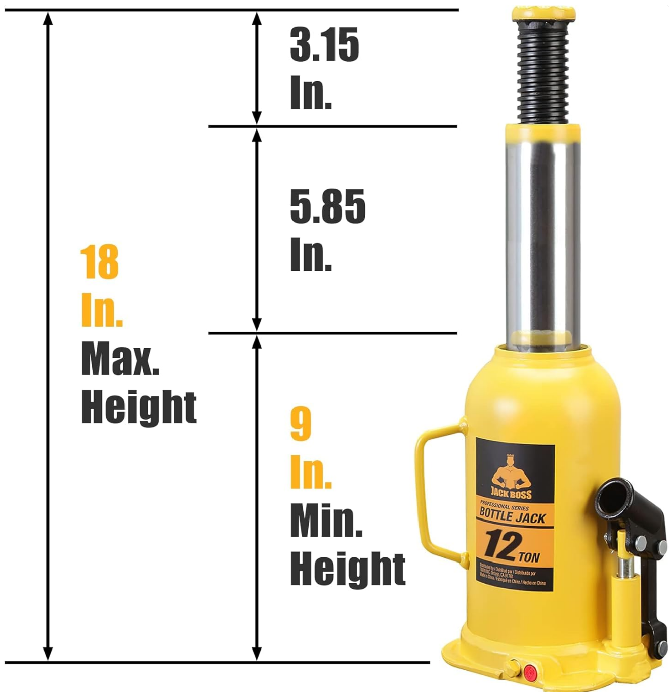
Figure 6: Detailed dimensions of the bottle jack, illustrating its minimum height (9 inches), maximum height (18 inches), and the adjustable screw top extension.
