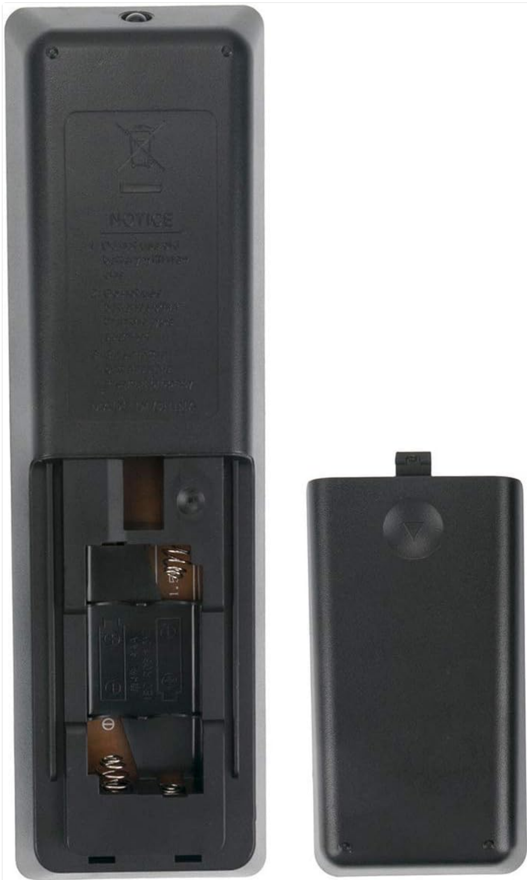
Image: Back view of the NH312UP remote control with the battery compartment open. This image shows the empty battery slots and the mechanism for opening the cover.
