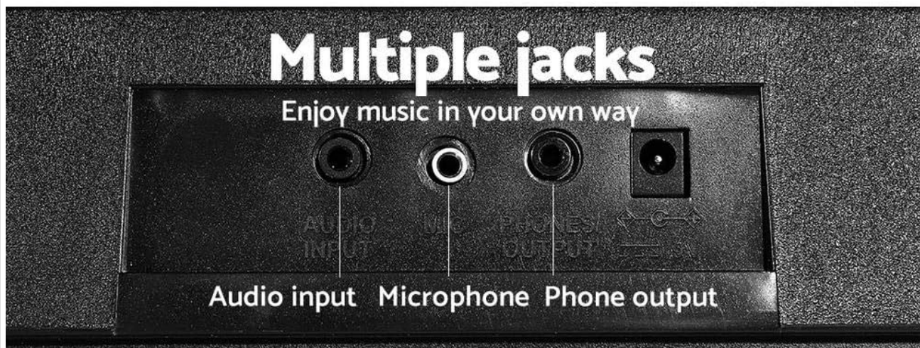
Figure 4.3: View of the multiple jacks including Audio Input, Microphone Input, and Headphone Output for versatile connectivity.
