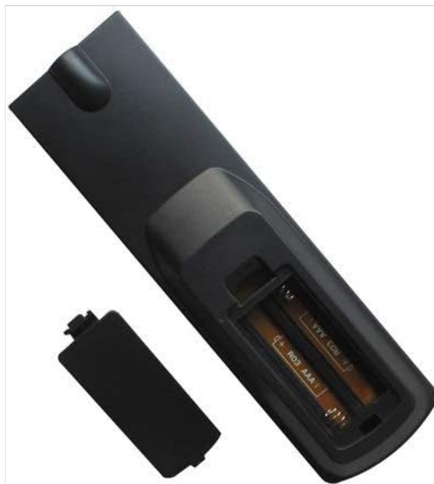
Image 2: Angled perspective of the remote control's back, showing the open battery compartment ready for two AAA batteries.
