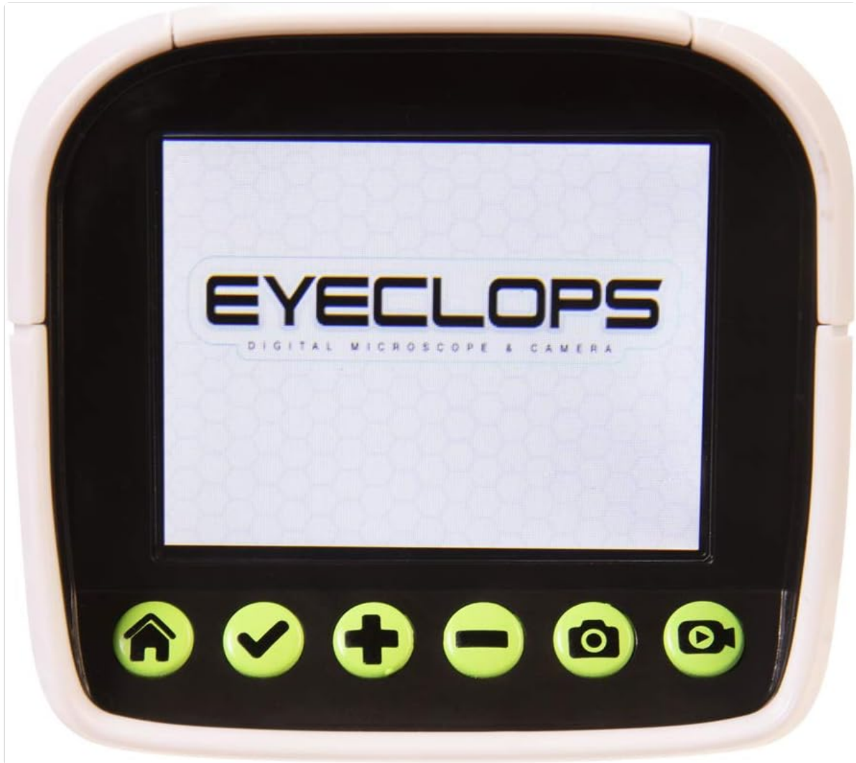
Image 4.1: A detailed view of the Eyeclops Digital Microscope's 2.4-inch color screen and its control buttons. The buttons typically include Home, Select/Confirm, Zoom In (+), Zoom Out (-), Camera, and Video functions.
