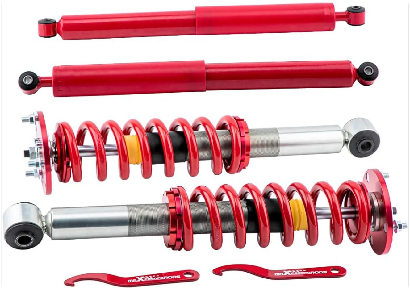
Image: A comprehensive view of the maXpeedingrods suspension kit, showing all four pieces: two front coilovers and two rear shock absorbers.
