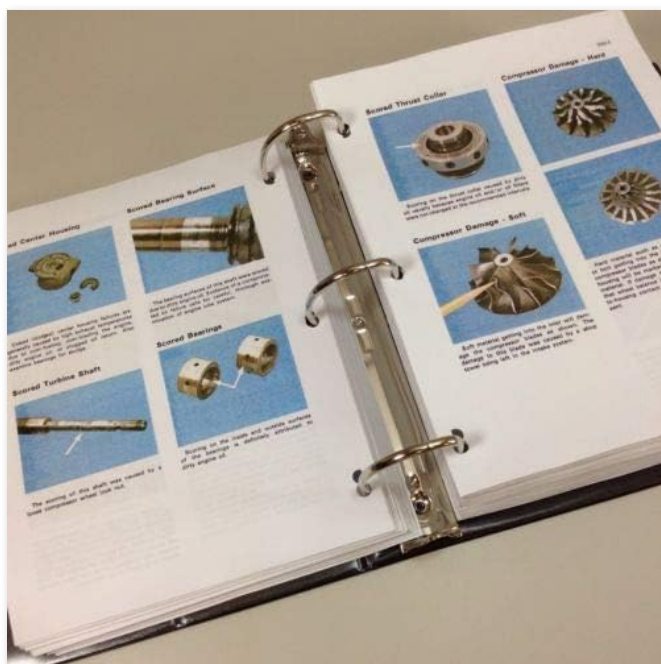
Figure 7: Example page providing visual examples of various types of compressor damage, useful for diagnostic purposes.
