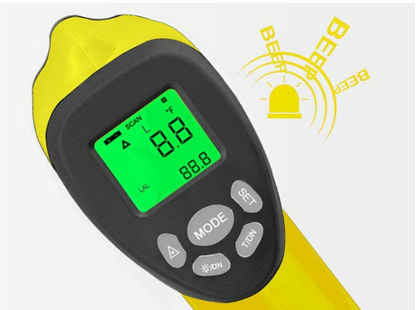
Figure 5.2: Display showing the High (H) and Low (L) temperature alarm indicators, which flash and beep when thresholds are exceeded.
