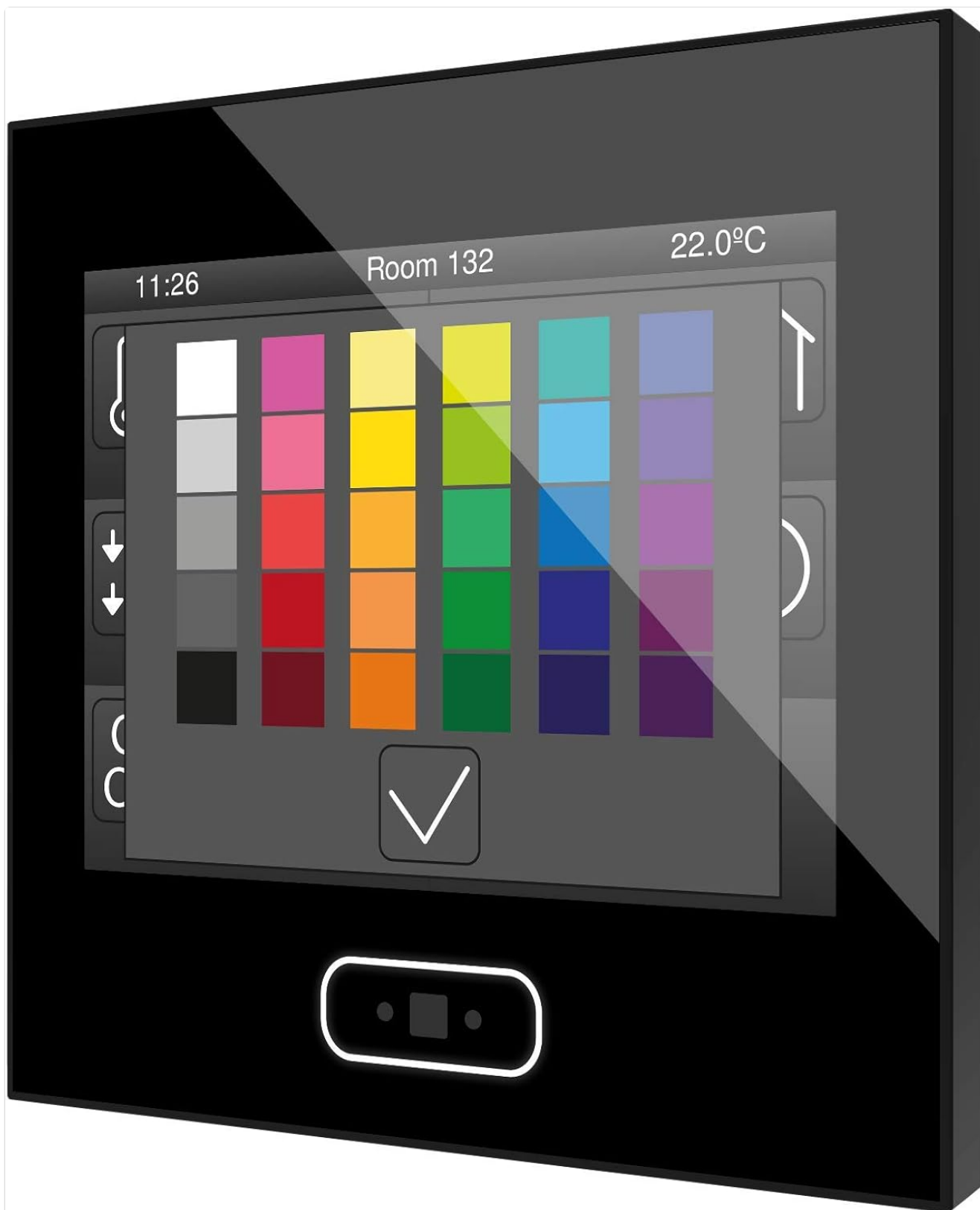
Figure 2.2: Front view of the ZENNIO ZVI-Z35-GW touch panel, illustrating the color selection interface. This feature allows users to choose specific colors, likely for RGB lighting control within the KNX system.
