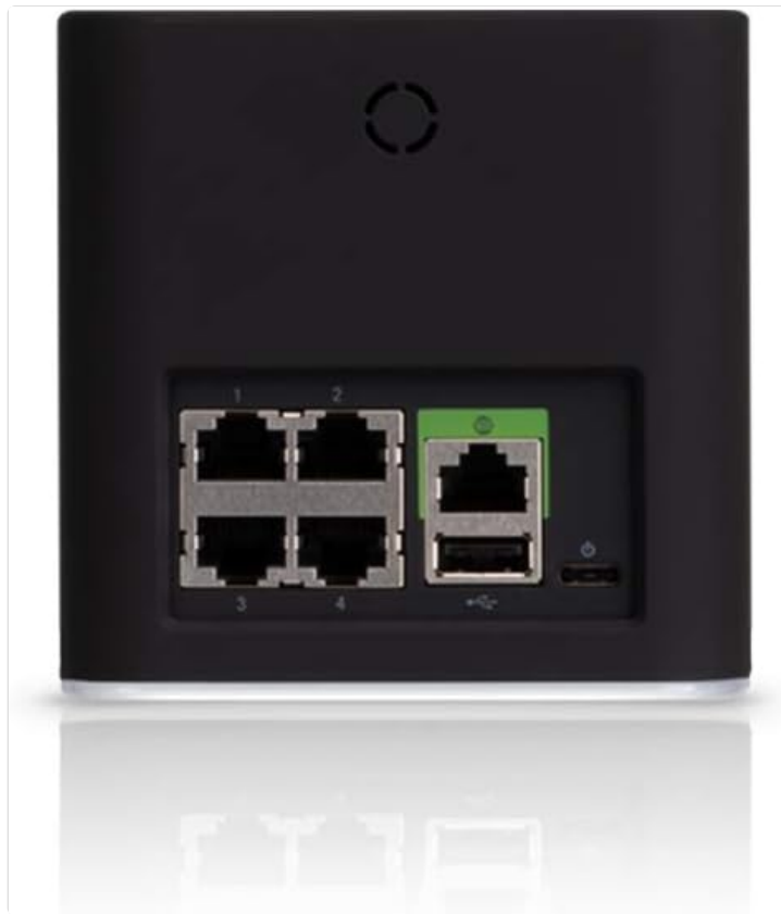
Image 3.1: Rear view of the AmpliFi router, highlighting the four Gigabit Ethernet ports and the WAN port.
