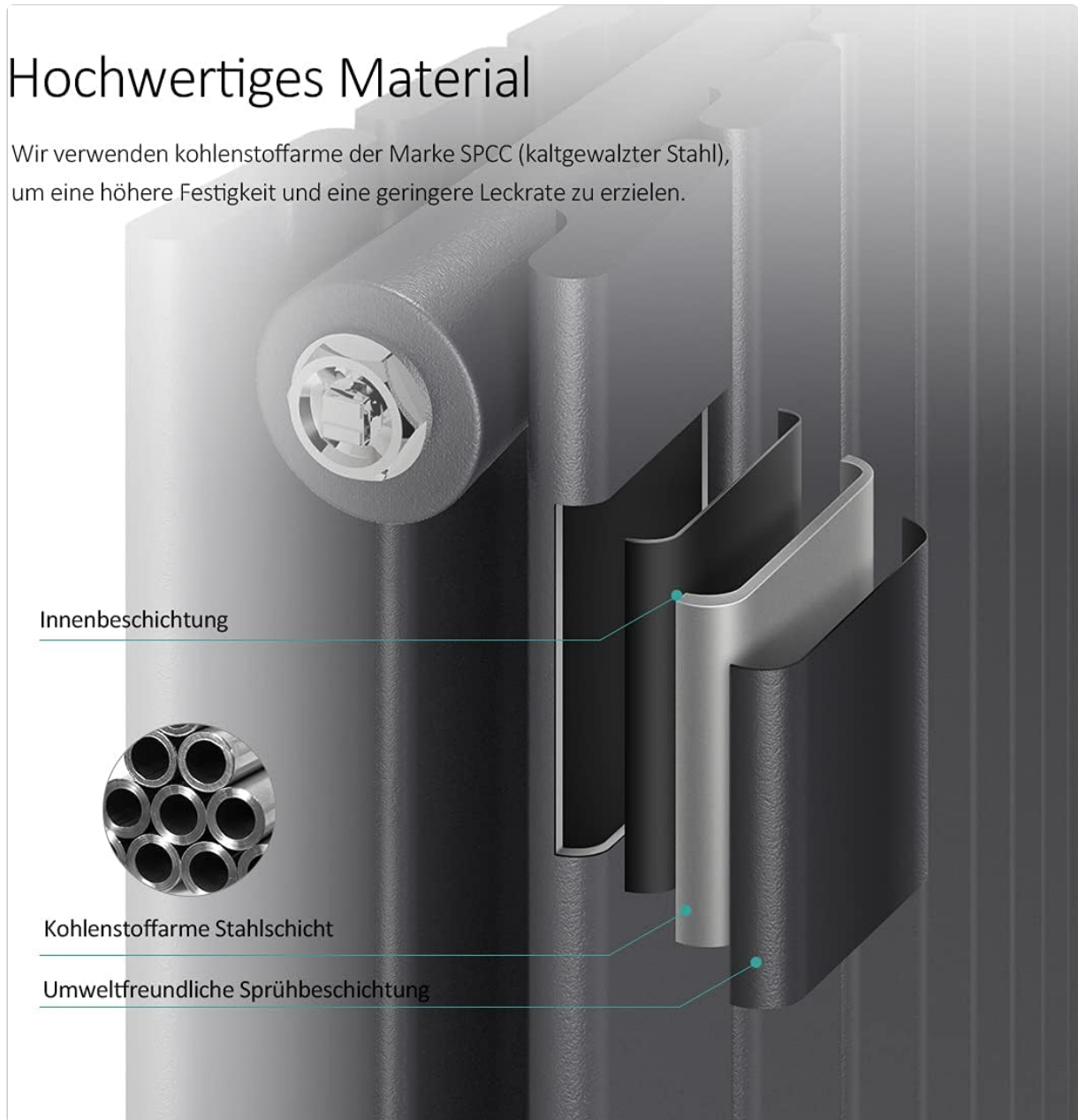
Image 5.1: Cross-section view highlighting the high-quality low-carbon steel, internal coating, and environmentally friendly spray coating.
