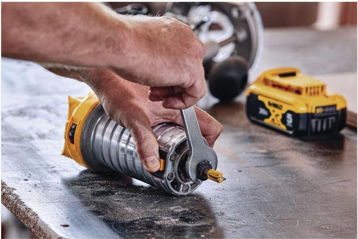
Image: A person using a wrench to tighten a router bit into the collet of the DEWALT router, ensuring it is secure.
