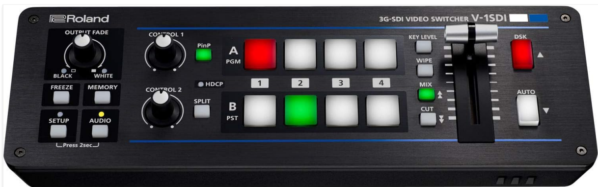
Figure 2.3: Top-down view of the V-1SDI control panel, highlighting the layout of buttons and indicators for program (PGM) and preview (PST) outputs.
