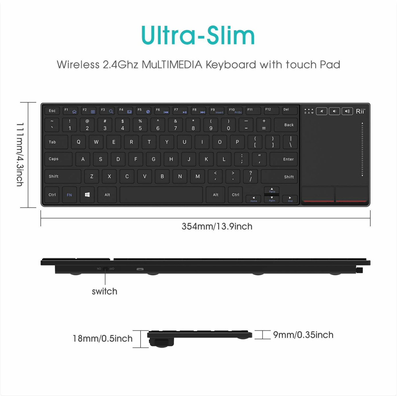
Figure 7.1: Rii K22 keyboard dimensions.
