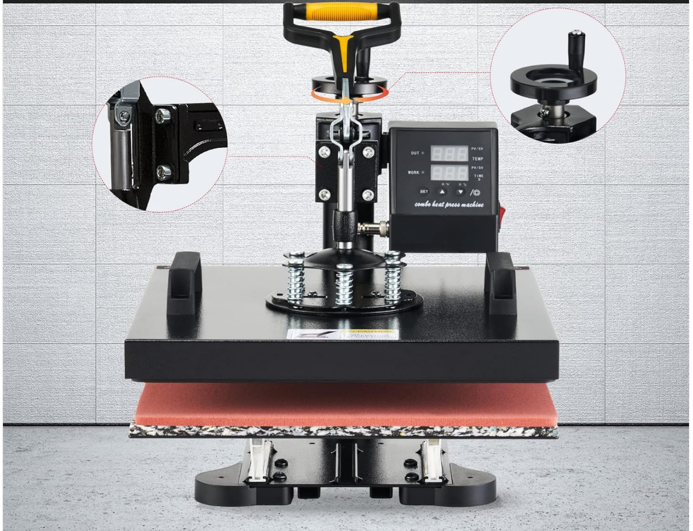
Figure 4.2: Easy Adjustment Knob for Pressure and Height
