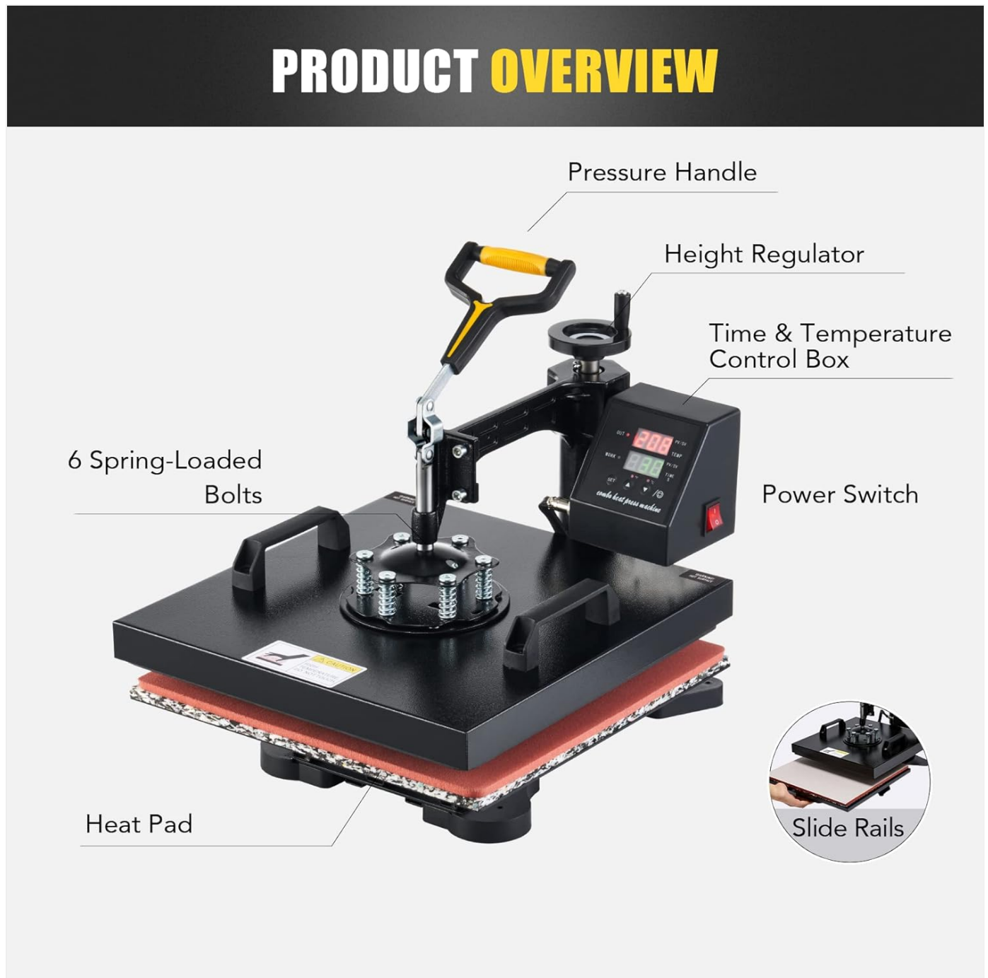
Figure 4.1: Main Components of the Heat Press Machine
