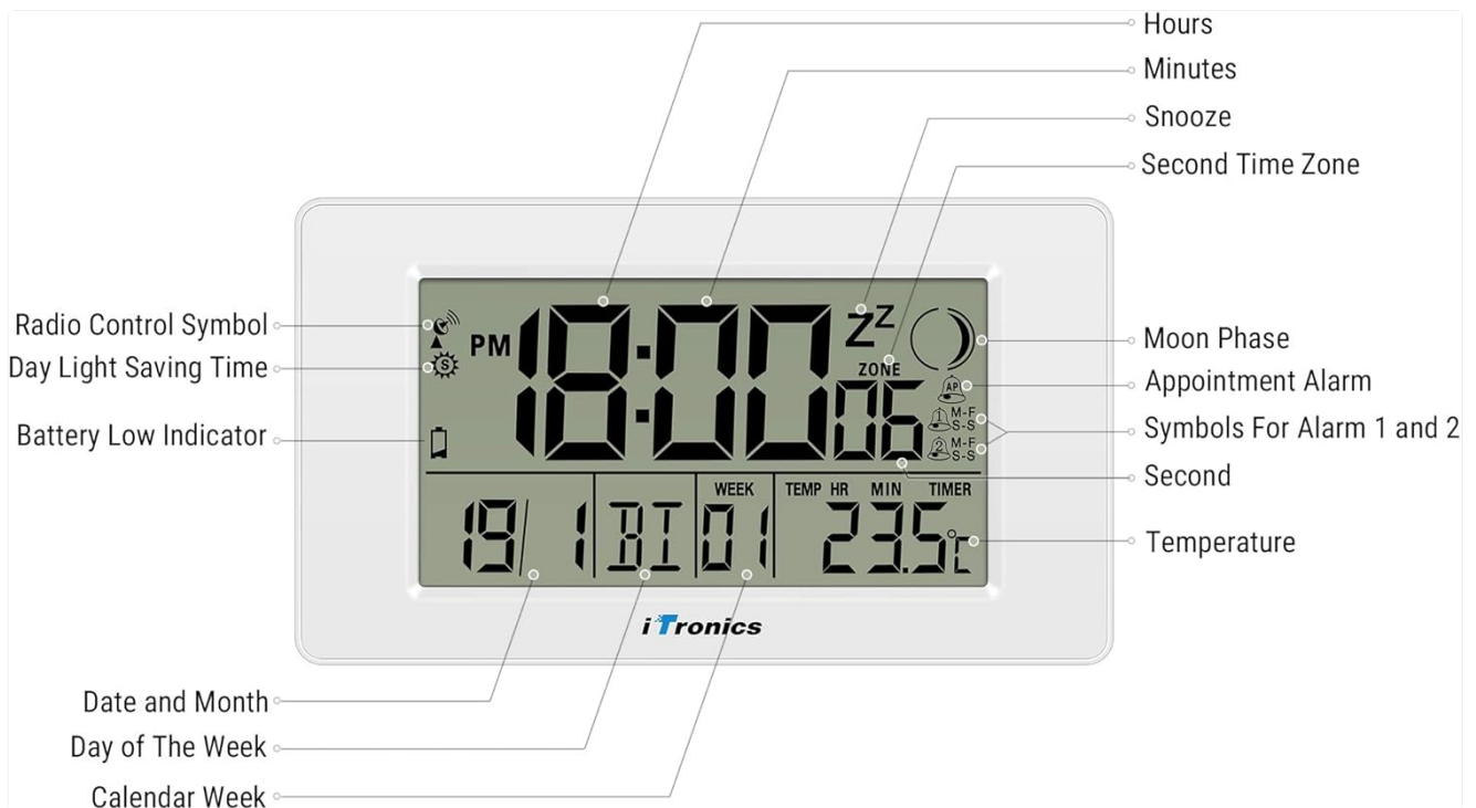
Image 5.1: Detailed diagram of the clock's display, indicating the position of the Radio Control Symbol, Day Light Saving Time, Battery Low Indicator, PM indicator, Hours, Minutes, Snooze, Second Time Zone, Moon Phase, Appointment Alarm, Symbols for Alarm 1 and 2, Second, Temperature, Date and Month, Day of The Week, and Calendar Week.
