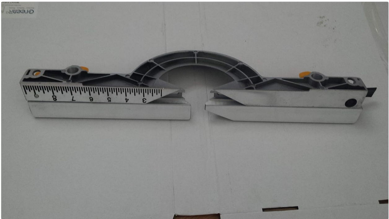
Figure 2.2: Detailed top view showing the ruler markings on the fence assembly.
