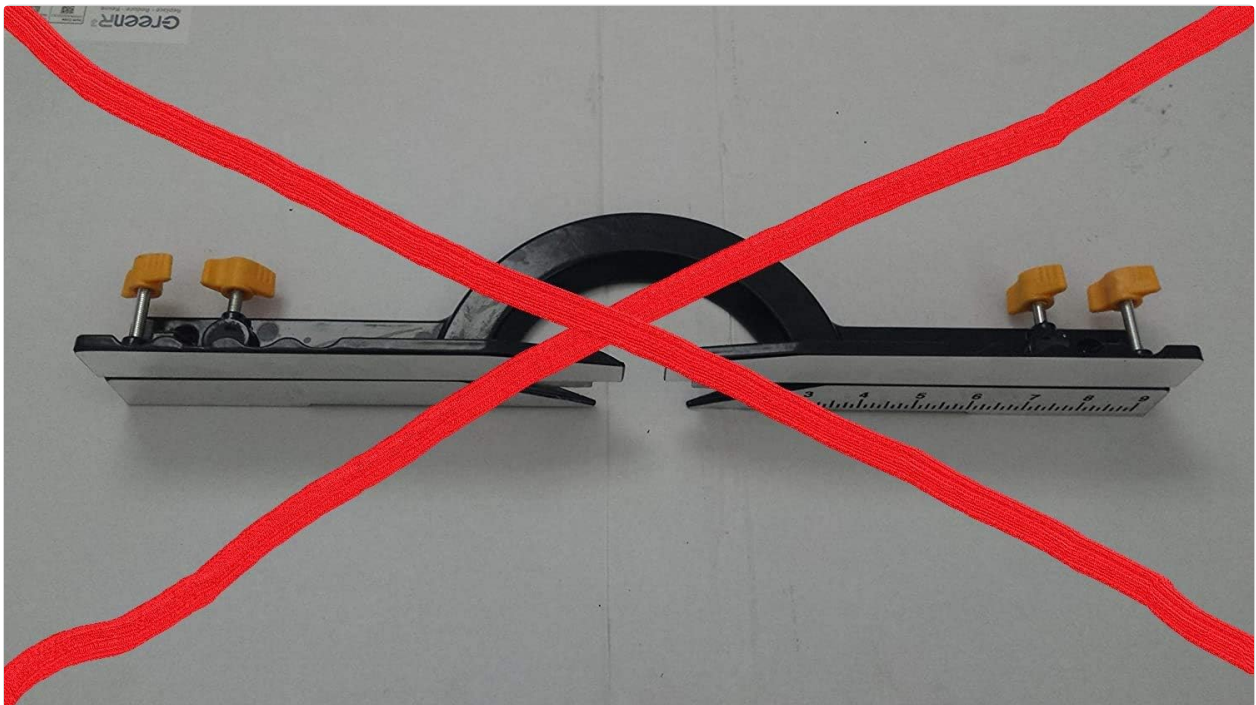
Figure 2.4: Example of an incompatible fence assembly (typically black). If your saw has a fence like this, this product will not fit.
