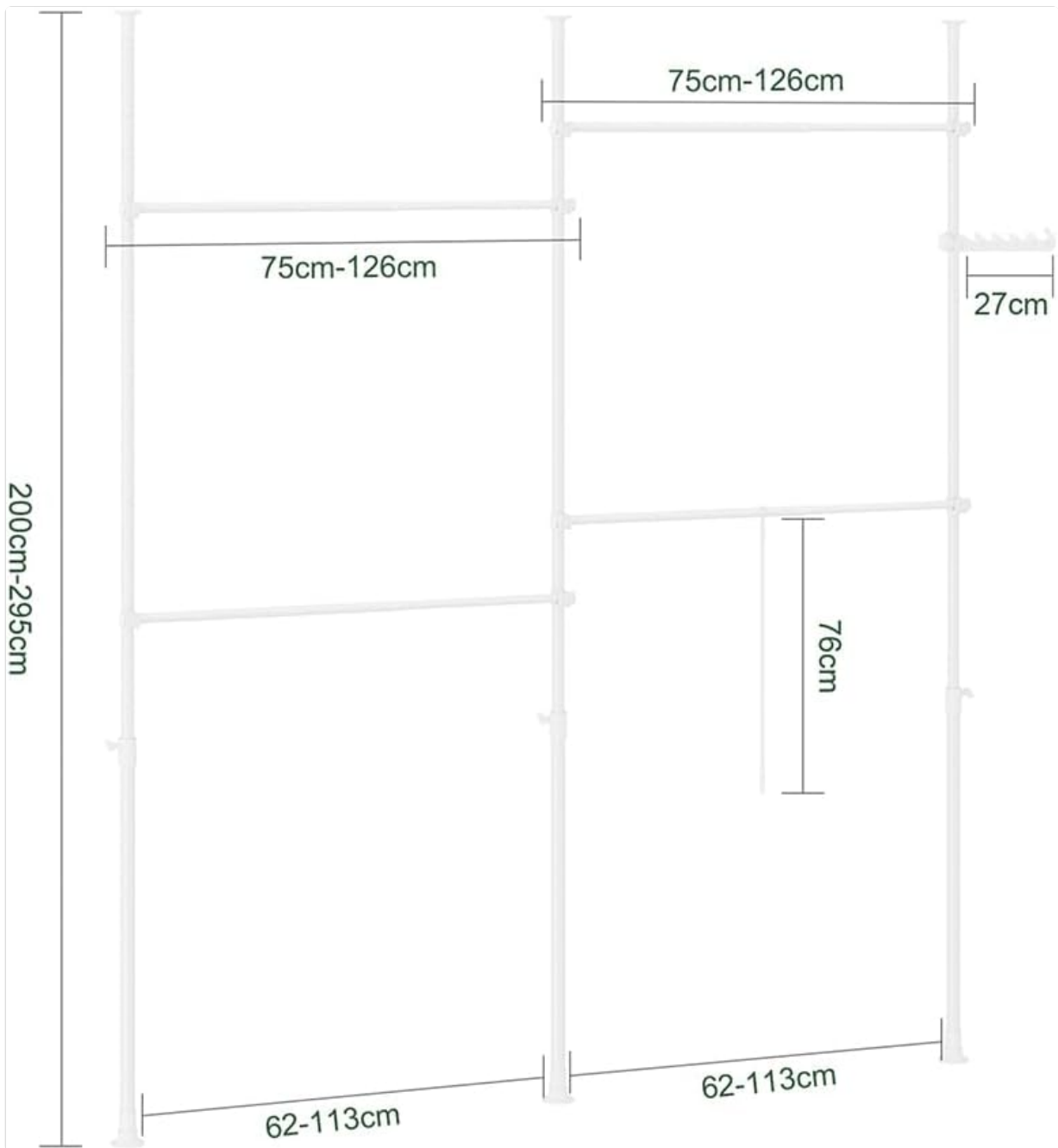
Image 3.3: Dimensional diagram illustrating the adjustable width and height of the garment rack, along with rod spacing.
