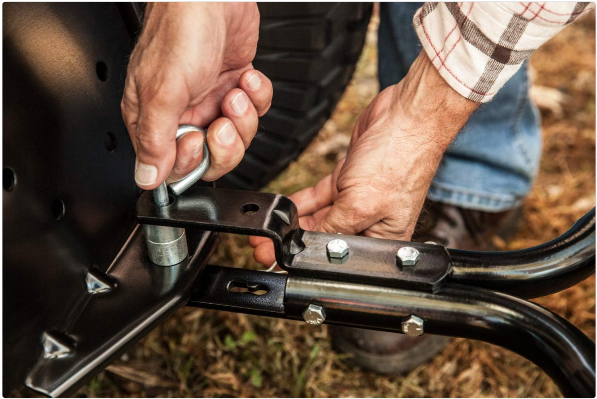
Image: Universal Hitch. This image shows the universal hitch mechanism, designed to connect the sweeper to various tractor models.
