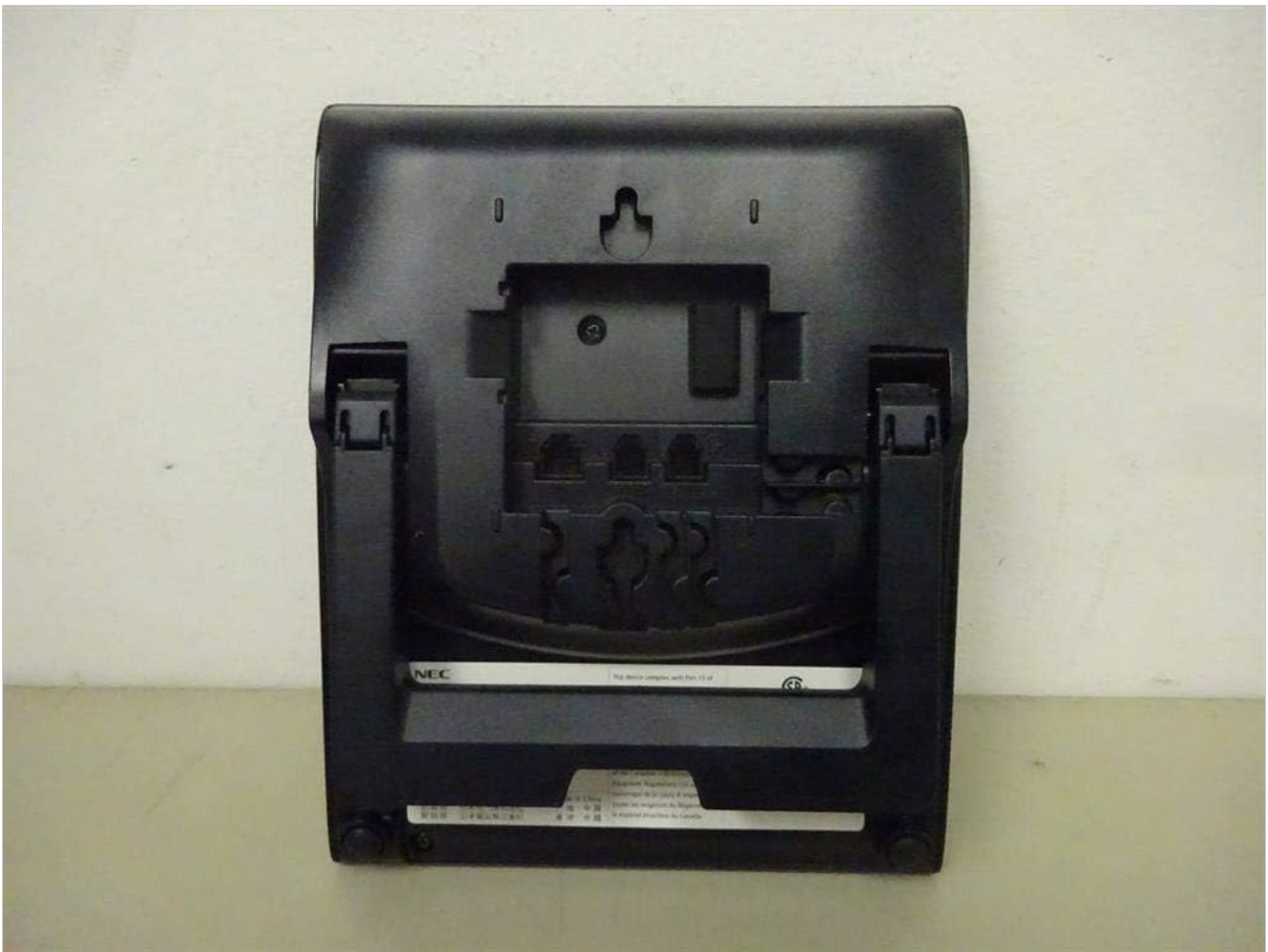
Figure 2: Rear view of the telephone, illustrating the various connection ports for the handset and network, as well as the integrated wall-mounting slots.
