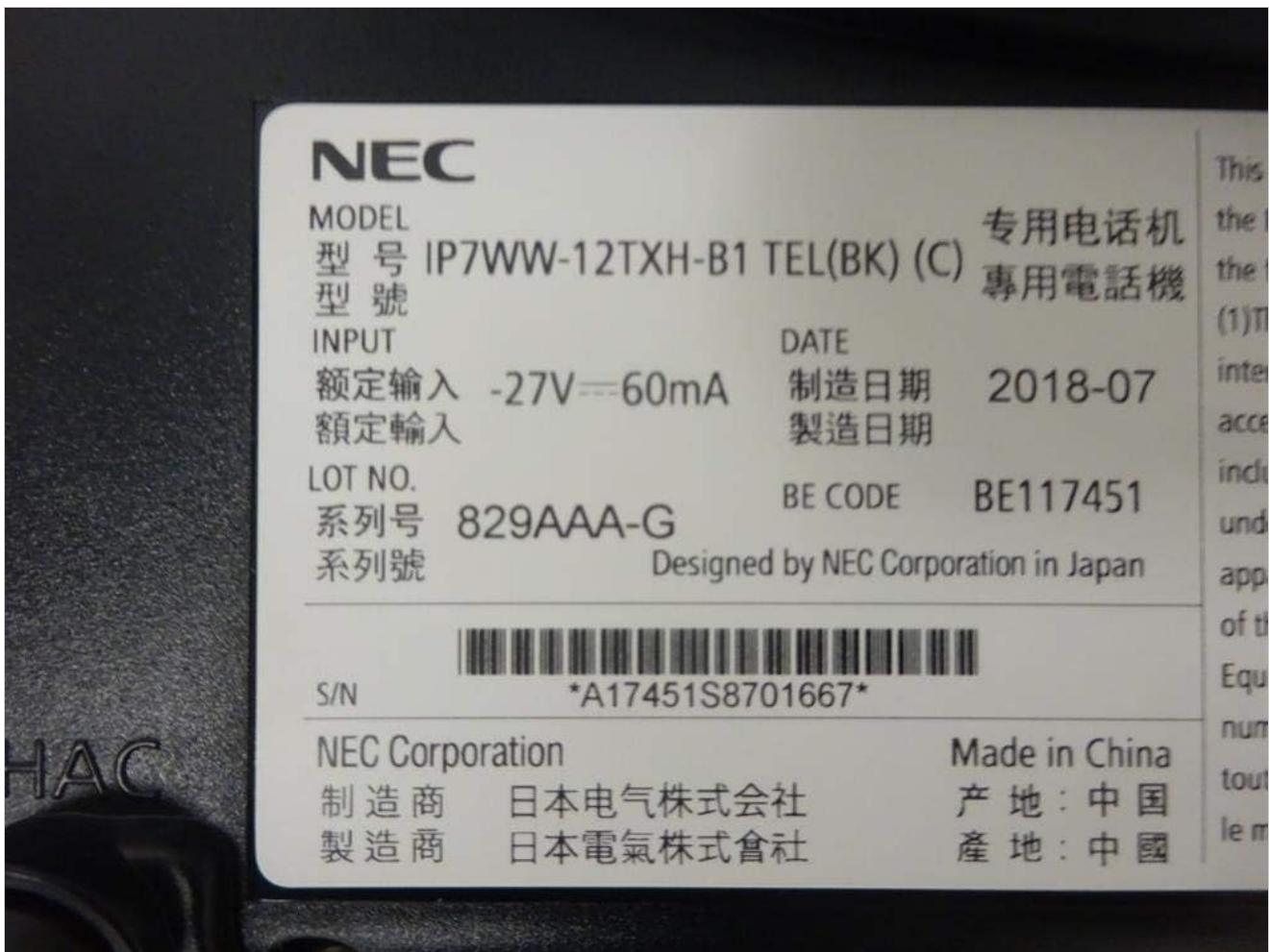
Figure 3: Close-up of the product label, displaying model number IP7WW-12TXH-B1, input specifications, and manufacturer details.
