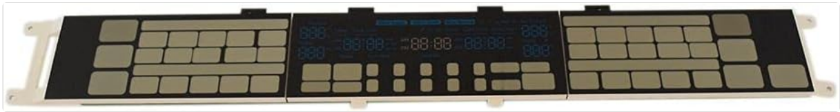
Figure 3.1: Front view of the Samsung DE92-04044B Electronic Control Board, showing the user interface and display area.
