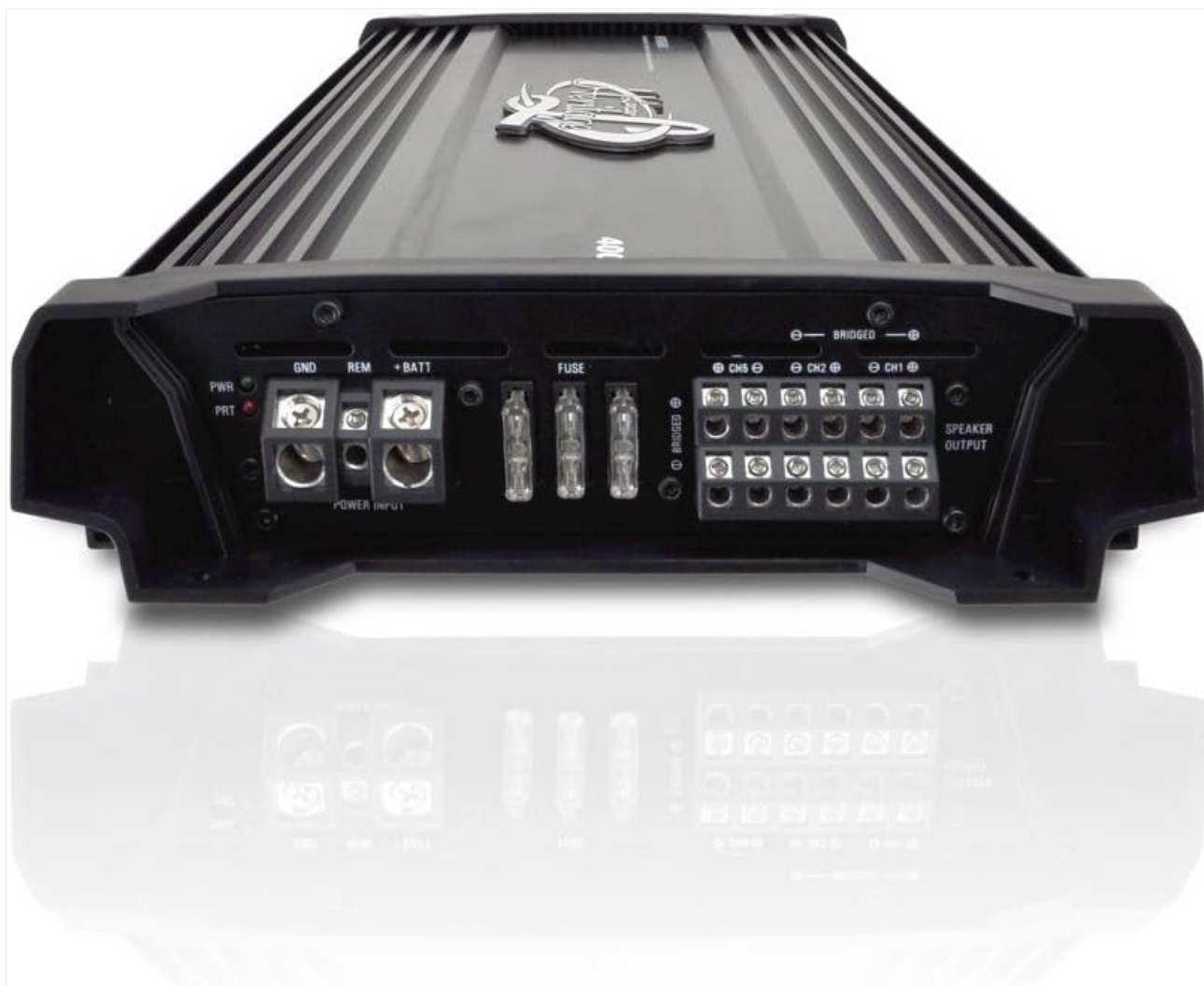
Image 5.2: Rear panel connections for power, ground, remote, and speaker outputs.
