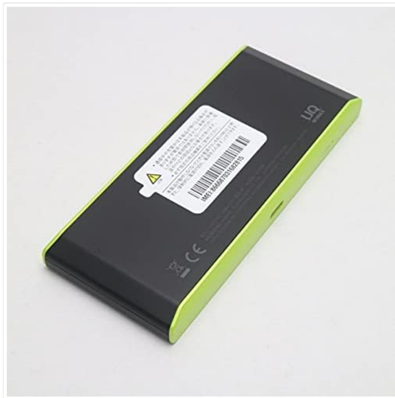
Figure 2.3: Rear view of the Huawei W05 mobile router, showing the product information label including IMEI and regulatory marks.
