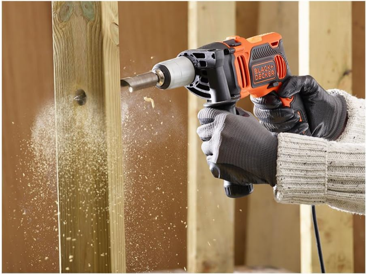
Figure 4: Drilling a large diameter hole in wood. Use appropriate drill bits and maintain control with the auxiliary handle.
