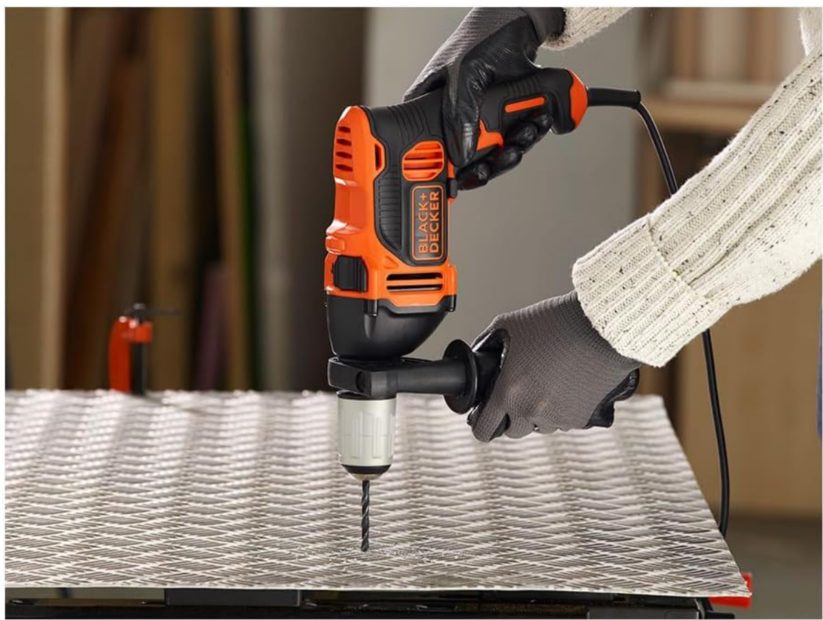
Figure 5: Drilling into a metal sheet. Ensure the workpiece is stable and use a suitable metal drill bit.
