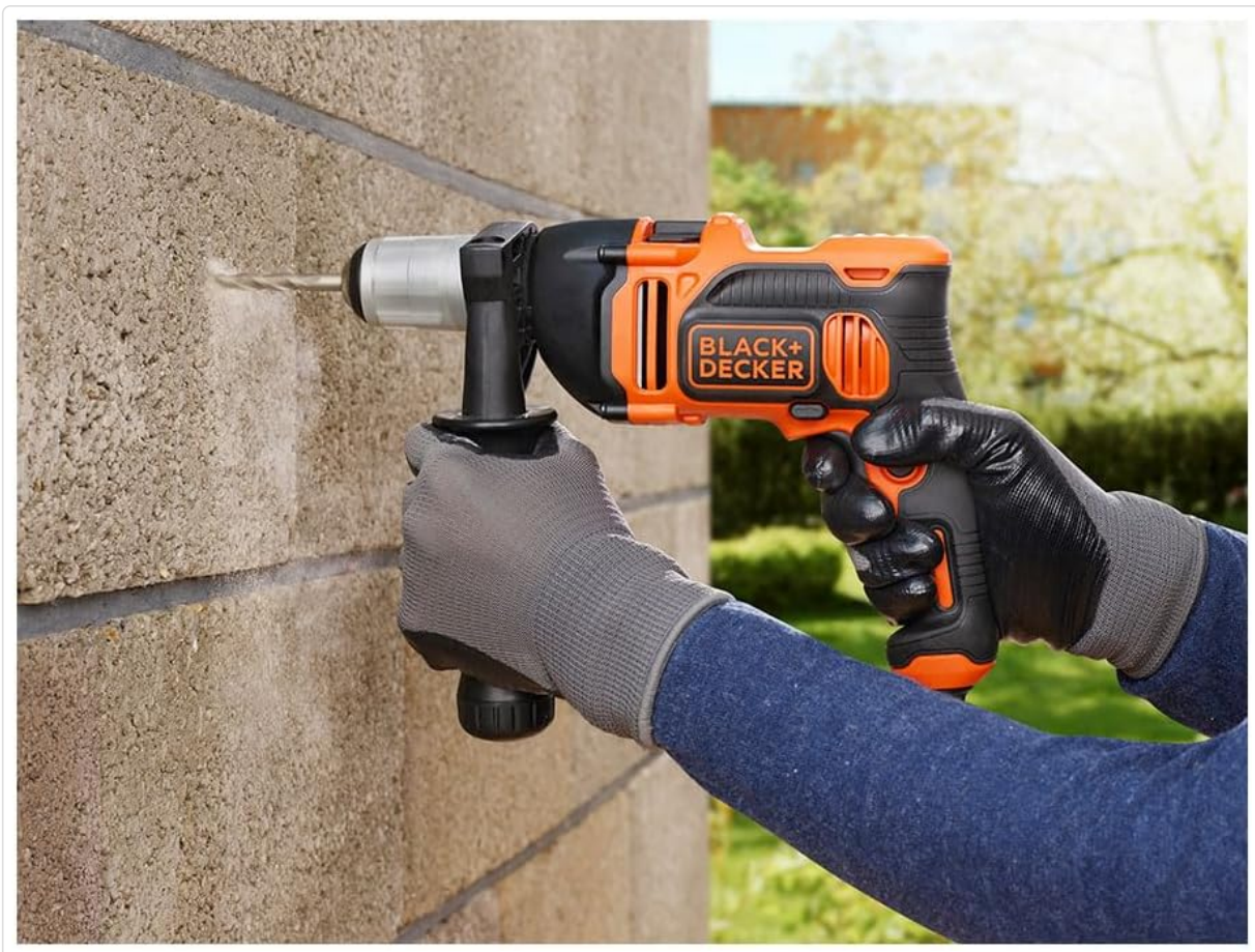
Figure 6: Drilling into a concrete block. Use hammer mode and a masonry drill bit for effective results.
